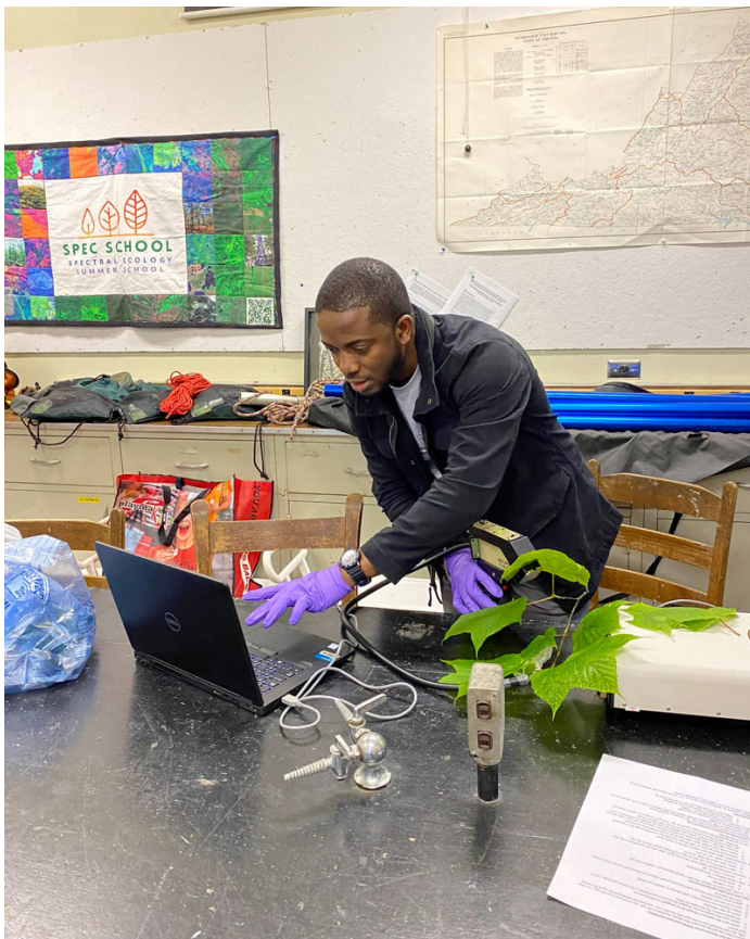
SPEC School participant Okikiola Michael Alegbeleye collects a leaf reflectance spectrum from a striped maple ( Acer pensylvanicum ) leaf using a Spectra Vista Corporation (SVC) spectrometer and leaf clip. (Image courtesy: Okikiola Michael Alegbeleye)
