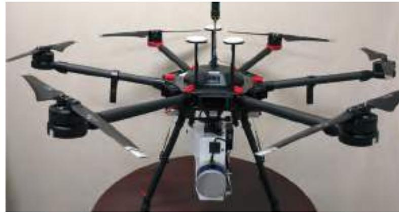
Headwall co-aligned hyperspectral / LiDAR autonomous system purchased as part of a Strategic Partnership Grant from MSU. This UAS will be used for plant phenomics research starting in the summer of 2020.
