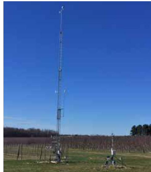
A twenty meter inversion tower installed in an apple orchard near Sparta, MI (left). This station is part of MSU's Enviroweather network ( https://www.enviroweather.msu.edu/ ).
