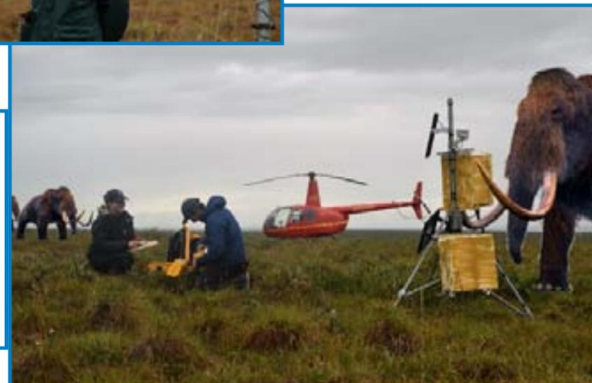
Right: Kelsey Nyland (left) and Clayton Queen (right) use DGPS equipment to collect highly precise measurements of ground surface subsidence at a CALM monitoring site on the Alaskan North Slope. Over an extended period the surface has been found to subside likely due to warming air temperatures.
