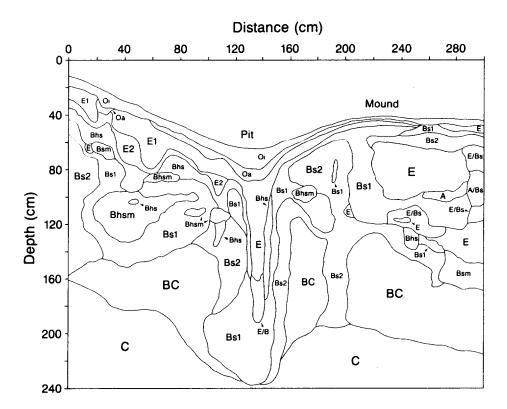
Fig. 1: Cross section through a pit/mound pair, illustrating deep tongueing of the E horizon in the pit. Soil horizon clasts are mixed in the center of mound, and do not reflect post-uprooting pedogenesis.
